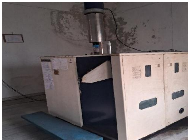
Fig. 2: Cobalt-60 Gamma Chamber 5000 for gamma irradiation treatment
